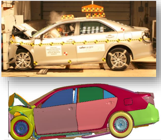
FIGURE 6 – Comparison of the Global Deformation for NCAP Test and Simulation
