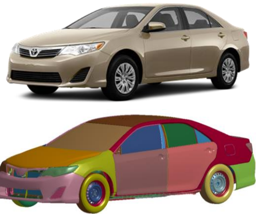
FIGURE 1 – Actual and FE Model of a 2012 Toyota Camry Sedan
